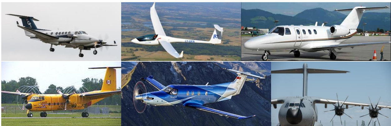
A Collage of T-Tails. Shown are, left to right, top to bottom: King Air, LS4 Glider, Citation 525, DHC-5, PC-12, A400M
