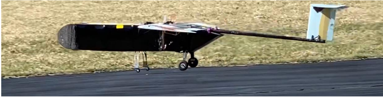
Shortly after take-off with minimal centerline drift (though still non-zero), and relatively flat liftoff despite elevator deflection
